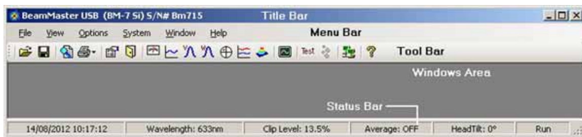
Figure 3-1. BeamMaster-USB Window Interface—Main Elements
