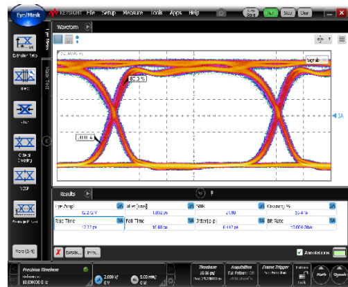
Output response Eye amplitude = 12.2 V pp
