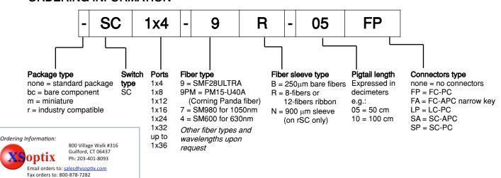
recalo's COAXIAL TYPE 1xN switch is non-latching: at power-off it breaks the optical connection and routing of the common port is not defined. The component is bidirectional, the common port can be used as input or output. The **PM Panda version** is offered up to 1x4 ports.
