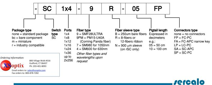
seregio's COAXIAL TYPE 1xN switch is non-latching: at power-off it breaks the optical connection and routing of the common port is not defined. The component is bidirectional, the common port can be used as input or output. The **PM Panda version** is offered up to 1x4 ports.
