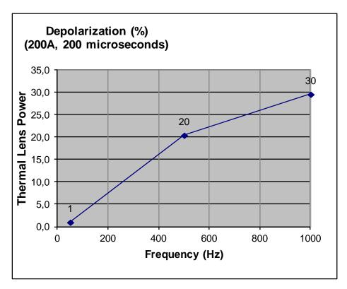
Typical QCW characteristics @ 1064 nm; output mirror pl: 85% reflection; back mirror pl; resonator length 140 mm.
