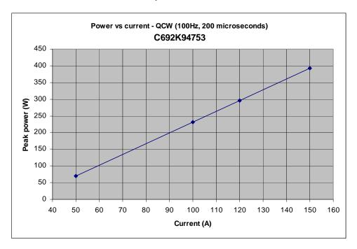
Typical QCW output @ 1064 nm; output mirror pl: 85% reflection; back mirror pl; resonator length 140 mm.
