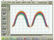
Optical Output Eye Diagrams - Demodulated 10 Gb/s CS-RZ-DPSK
