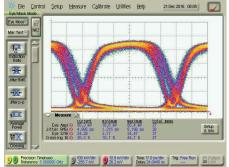
Optical Output Eye Diagrams - 10 Gb/s RZ-DPSK
