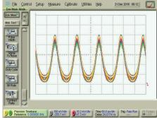
Optical Output Eye Diagrams - 10 Gb/s Demodulated RZ-DPSK
