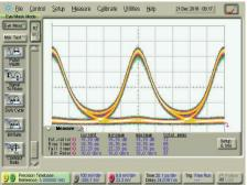
Optical Output Eye Diagrams - 10 Gb/s CS-RZ-DPSK
