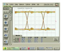
Input signal Eye amplitude =  $0.5 \, V_{pp'}$  Rise time = 9 ps Jitter RMS =  $309 \, fs$ , SNR = 41
