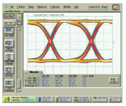
Output response Eye amplitude =  $6 V_{pp'}$  Rise time = 12.67 ps Jitter RMS = 934 fs, SNR = 26
