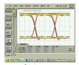
Output response Eye amplitude =  $7.3 \, V_{pp'}$  Rise time =  $12.4 \, ps$ Jitter RMS =  $712 \, fs$ , SNR = 37.5
