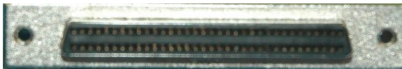
Figure 9 Photograph of the auxiliary control port on the SV1C.
