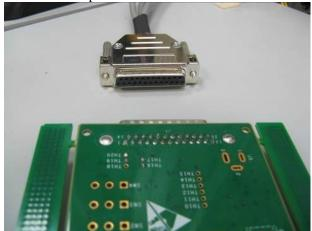
4. Connect the 30-pins connector (J3) with the EDFA module's 30-pins connector
