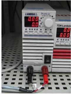
a. The power supply plugs (+5V – denoted by red color, and GND – denoted by black color) must be connected to 5V DC power supply source.
