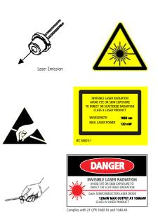
Unpacking the laser diodes should only be done at electrostatic safe workstations (EPA). Though protection against electro static discharge (ESD) is implemented in the laser package, charges may occur at surfaces. Please store this product in its original package at a dry, clean place until final use. During device installation, ESD protection has to be maintained.
