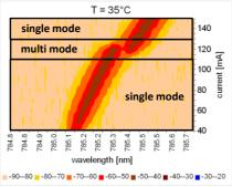
The spectral maps show the power spectral density at different operating modes. The graphs illustrate that the laser exhibits single and multi mode behavior under different operational conditions. The spectral maps may differ from part to part. Single mode operation can be achieved by selecting the appropriate laser current and temperature.
