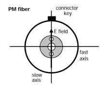
slow axis of the PM fiber aligned to connector key
