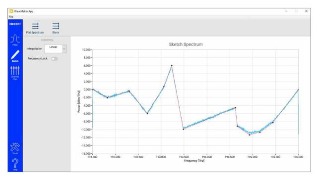
A signal with an arbitrary spectral shape can be defined by drag-and-drop using the mouse of the PC, as shown with the red curve in the screenshot above. The created shape will immediately be uploaded to the WaveMaker. The output spectrum, measured with the internal Optical Spectrum Analyzer module, is shown with the blue trace.
