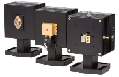
The 240 Series LaserMounts support C-Mount, HHL, and TO-3 devices for high performance and long term operation. All mounts feature solderless connections and an integrated fan for maximum thermal performance. Each fixture includes a removable pedestal, and is easily mounting to an optical table.
